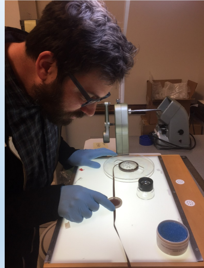
Using the lightbox of the rewind to see audiotape track configuration
