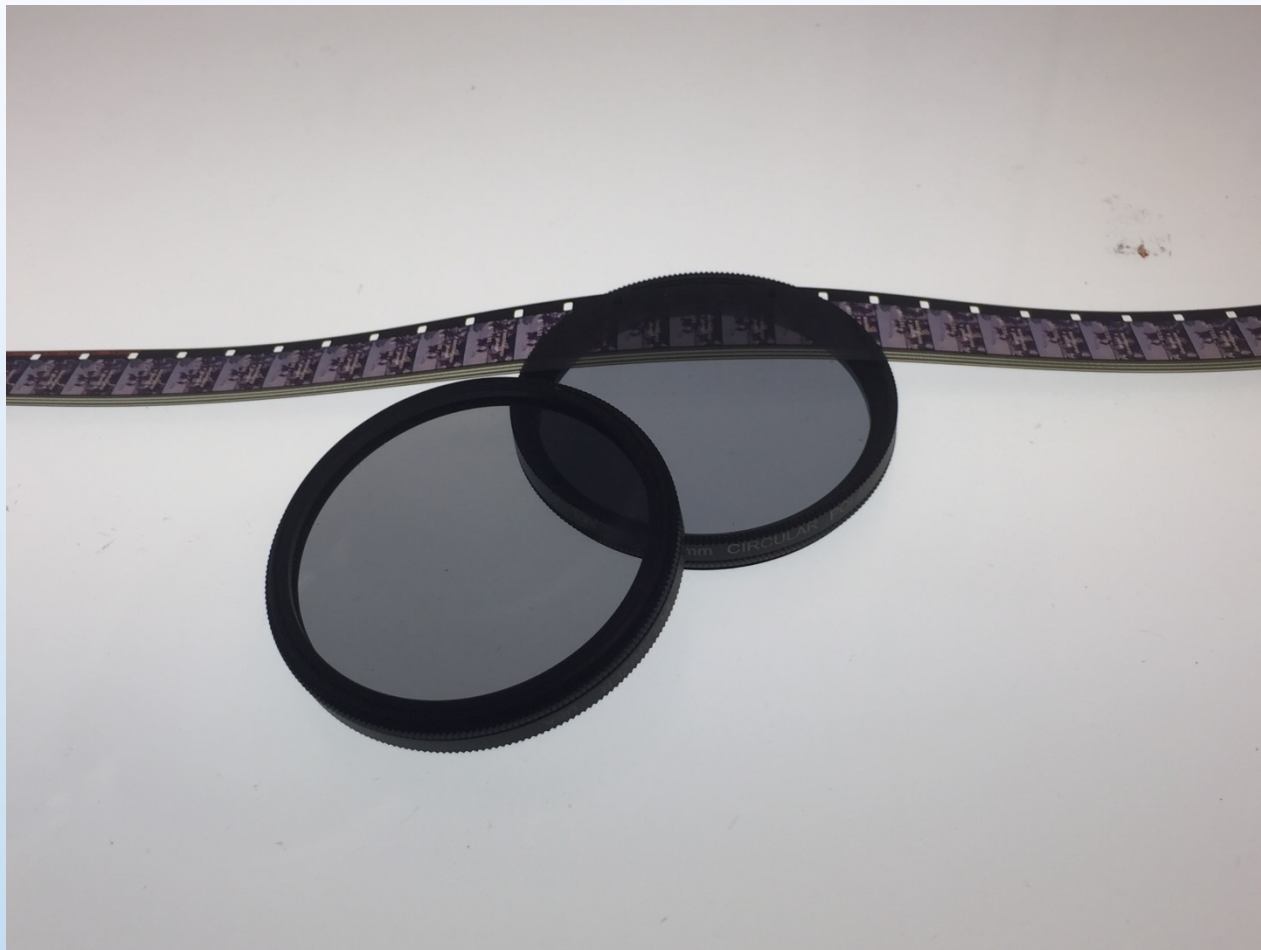
Polarized Lenses to distinguish nitrate/acetate bases from polyester
