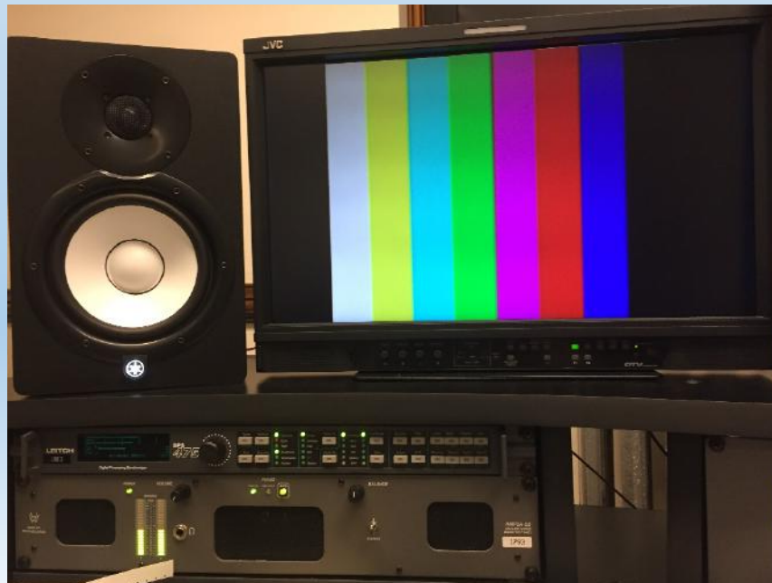
Speaker (left), Video Monitor (Right), Time- Based Corrector a. k. a Frame Synchronizer (bottom)
